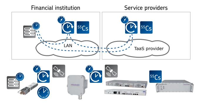
OSA 5401 SyncPlug<sup>™</sup>: SFP-based on-site PTP grandmaster OSA SoftSync: NTP/ PTP software client OSA 5405 SyncReach™: Onsite gandmaster with integrated dual-GNSS receiver OSA 5420/30: Edge/core grandmaster featuring various oscillator options, NTP gateway, 1/10 GE OSA 3235B: Optical atomic cesium clock for longest holdover
